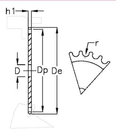
C = 1 D = 16 De = 140.7 Dp = 136.54 For chain size = 3/8 x 7/32 For chain type = 06 B-1 h1 = 5.3 Sumber of teeth = 45
